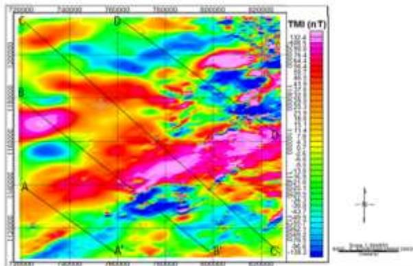
Fig. 4. Residual map of the study area with profiles A-A', B-B', C-C' and D-D' used in modeling.
